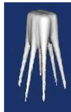
An isotherm around a ground thermal storage facility using multiple slanted bore holes. Computed in 3D using IDA ICE.
